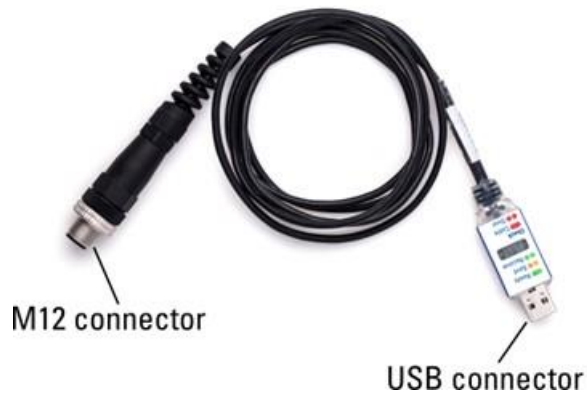
Figure 2 The connectors of the Smart Interface Cable.
