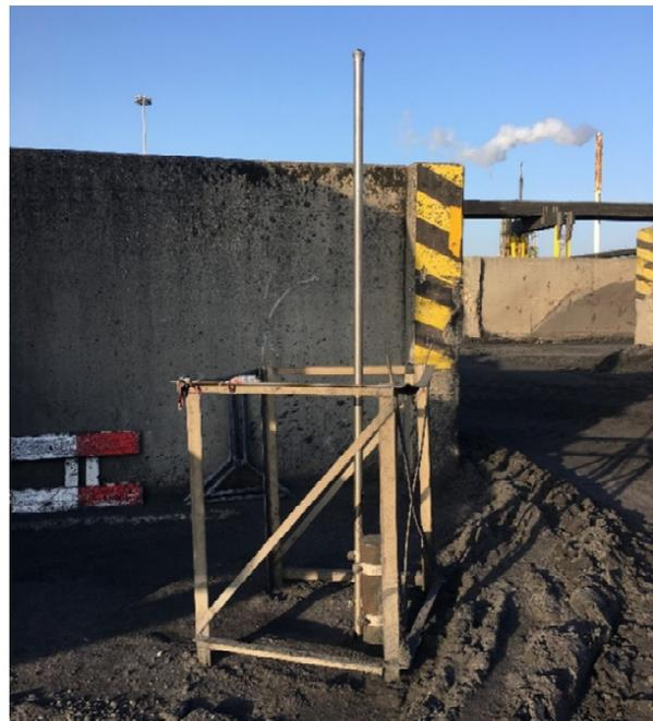
Monitoring well with Diver-DXT radio module placed on a 3-meter high pole next to the well (source: ESD-SIC)
